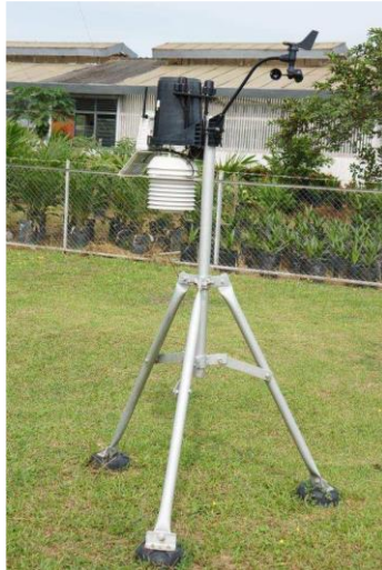
Gambar 3.8 Automatic Weather Station
